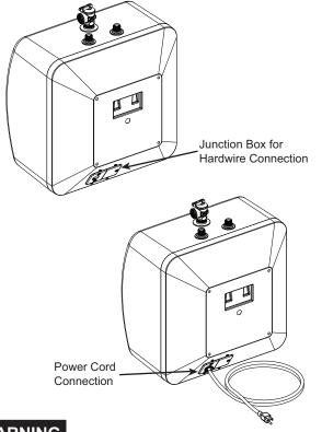
AWARNING Proper ground connection is essential. The presence of water in the piping and water heater does not provide sufficient conduction for a ground. Nonmetallic piping, dielectric unions, flexible connectors, etc., can cause the water heater to be electrically isolated. Do not disconnect factory ground.
