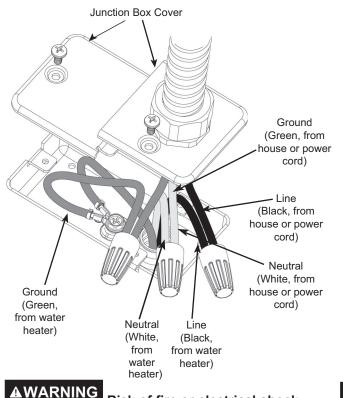
**A WARNING** Risk of fire or electrical shock. Ensure both junction box covers and ground screws are securely fastened for proper grounding.
