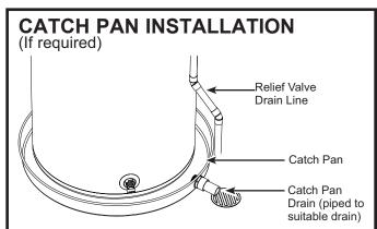
**NOTE:** Auxiliary catch pan MUST conform to local codes. Catch Pan Kits are available from the store where the water heater was purchased, a builder store or any water heater distributor. The catch pan should be 2" (5.1 cm) minimum larger than the Water Heater base diameter. To prevent corrosion and improve Drain Valve access it is recommended that the water heater be placed on spacers inside the catch pan.
